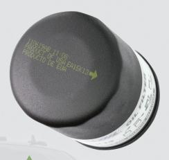
AMSOIL Oil Filters feature a reference arrow to aid in proper installation. Once the filter is finger tight, it is easy to gauge the additional three-fourths to 1.25 turns required to ensure a good fit. Over-tightening can lead to leakage.
